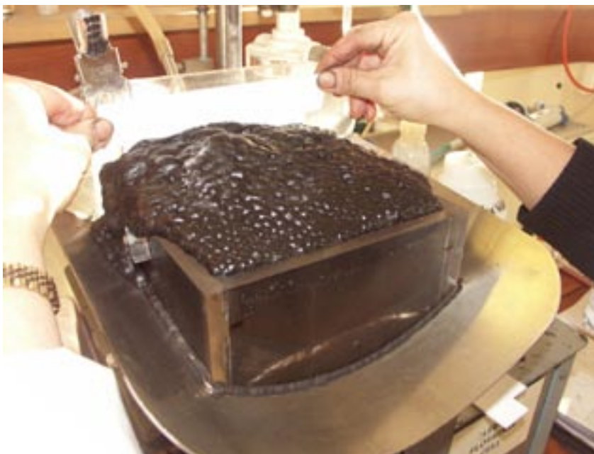
Froth flotation test in progress in CRL Energy's coal preparation laboratory. Photo: Trevor Dine.
