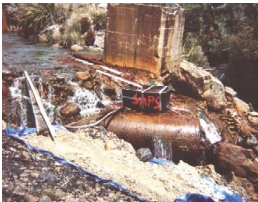
A range of remediation systems were tested including anoxic and oxic limestone drains, and successive alkalinity producing systems which were particularly positive.
